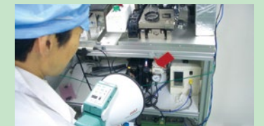
Air leakage is measured at designated checkpoints
